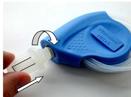
4. Screw the closure cap back into place as far as it will go into the spiral unit.
