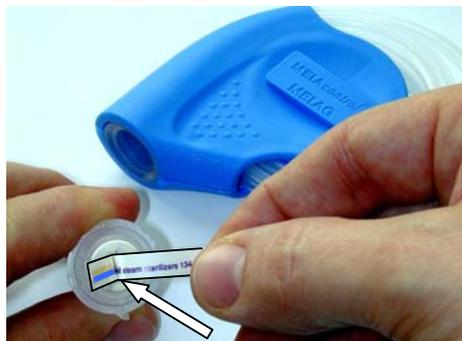
3. Insert the middle fold of the **indicator strip** into the closure cap of the spiral unit. Insert the indicator strip as far as it will go into the cap.
